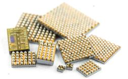
package footprint reductions, lower cost, improved electrical performance, and a relatively simpler construction over conventional wirebond or interposer packaging technologies.
