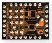
Passive devices such as resistors, capacitors, inductors, filters and baluns can consume 60-70% of available space in a system, subsystem or SiP. As one of the first companies in the industry to integrate and fabricate passive devices at the silicon wafer level, we are able
